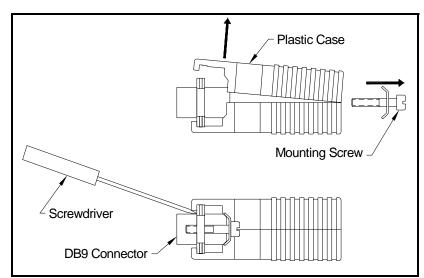
Figure 6-2: Opening the Converter Case
