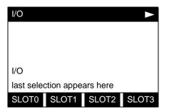
Use the  $[\leftarrow]$  and  $[\rightarrow]$  and the [F1]-[F4] keys to select the desired slot number. (Only those slots which contain an option card will appear on the option bar.)
