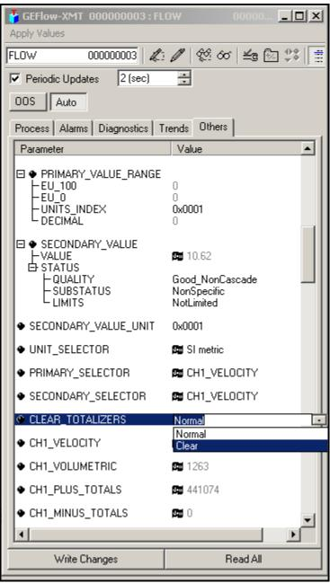
Figure D-4: Clear Totalizers Drop Down List
