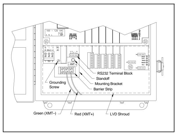
Figure 6-1: Interface Converter Mounting
