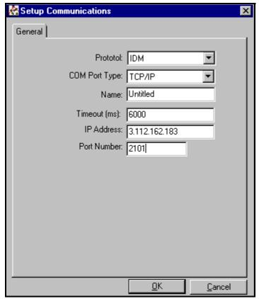
Figure C-3: Setup Communications for TCP/IP
