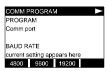
To change the baud rate, press the  $[\rightarrow]$  key until the desired baud rate appears on the option bar, and then press the appropriate [Fx] function key.
