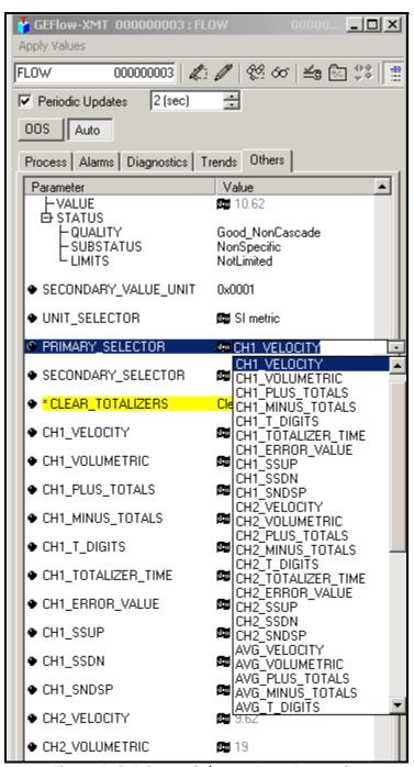
Figure D-2: Primary Selector Drop Down List
