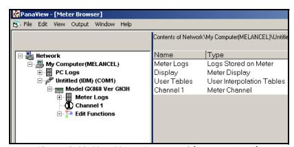
Figure C-18: New Meter Browser with Meter Branch
