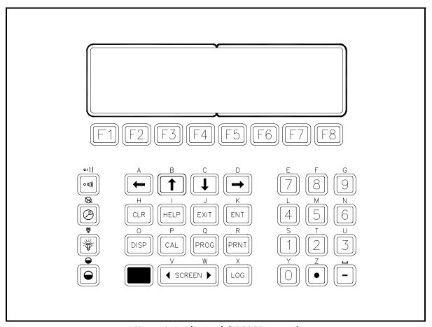
Figure 1-1: The Model GC868 Keypad
