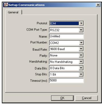
Figure C-2: Setup Communications Screen
