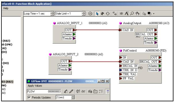
Figure D-5: Function Block Application
