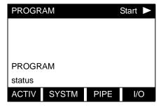
Press the  $[\leftarrow]$  and  $[\rightarrow]$  keys and one of the function keys [F1]-[F4] to select the desired submenu. From this screen, press [EXIT] to return to measurement mode.
