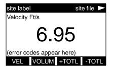
Use the [F1]-[F4], [ $\leftarrow$ ] and [ $\rightarrow$ ] keys to select the desired display parameter option. See Table 2-1 below for a complete description of the available options.
